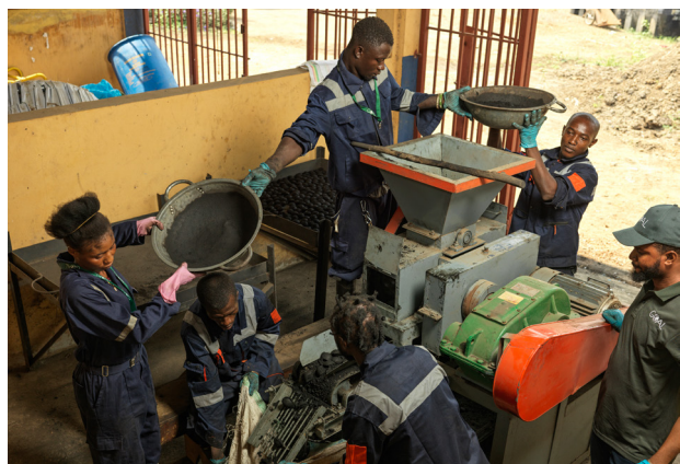
Workers at ICSP and GOAL-supported Waste to Energy plant adding the prepared mix into the briquette forming machine © GOAL
