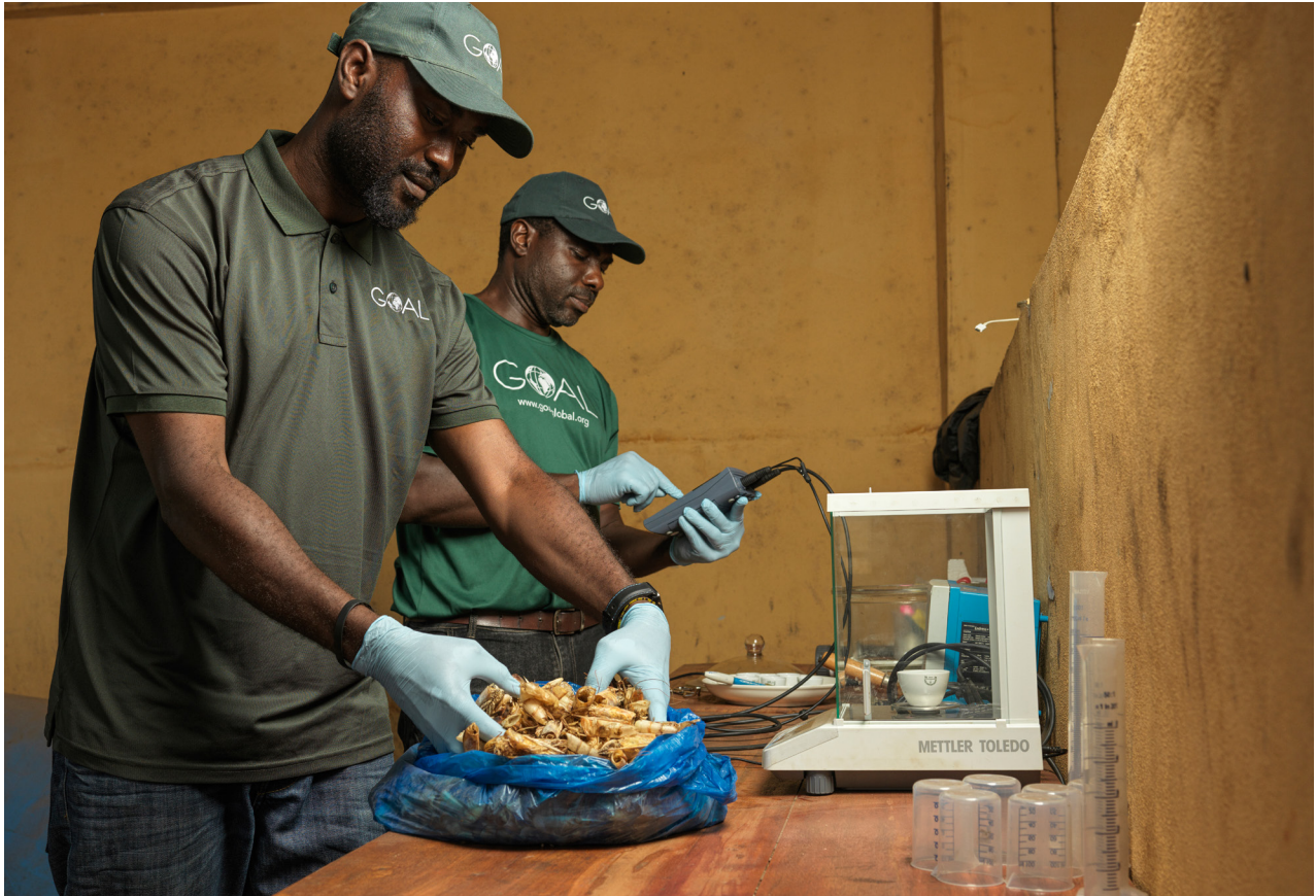
Shrimp shells are ground & added to dried biomass mix during production of briquettes, creating a low-cost and smokeless alternative to charcoal © GOAL
